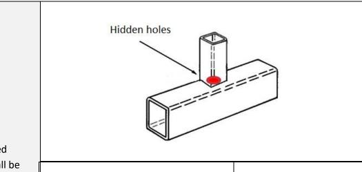
The concealed openings shall be selected and arranged so as to ensure smooth pull-out from the sump and the least possible zinc residue inside the structure
