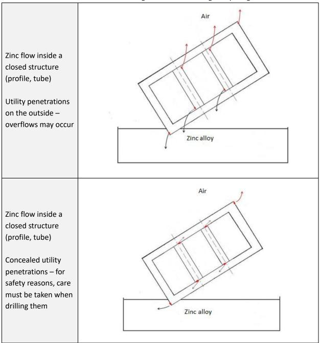
TABLE 2 – Design of openings. The required size of the following openings also applies to the size of the external openings.
