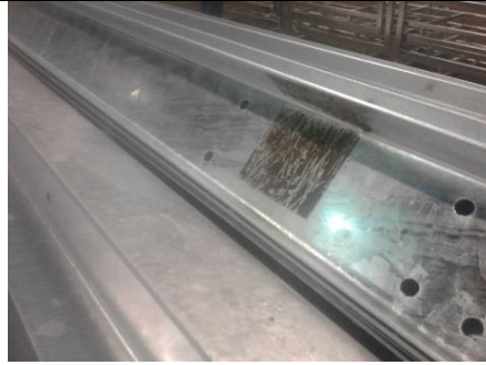
Impurities on steel, sticker marks resulting in lack of zinc plating – remain unpainted
