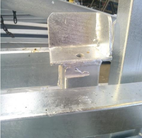
Impurities on steel, sticker marks resulting in lack of zinc plating – remain unpainted
