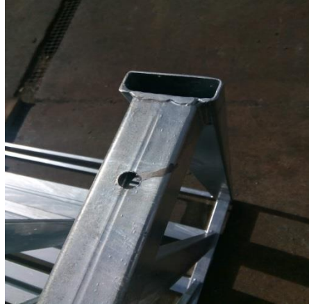
Sling (wire) marks, ash marks – are not treated
