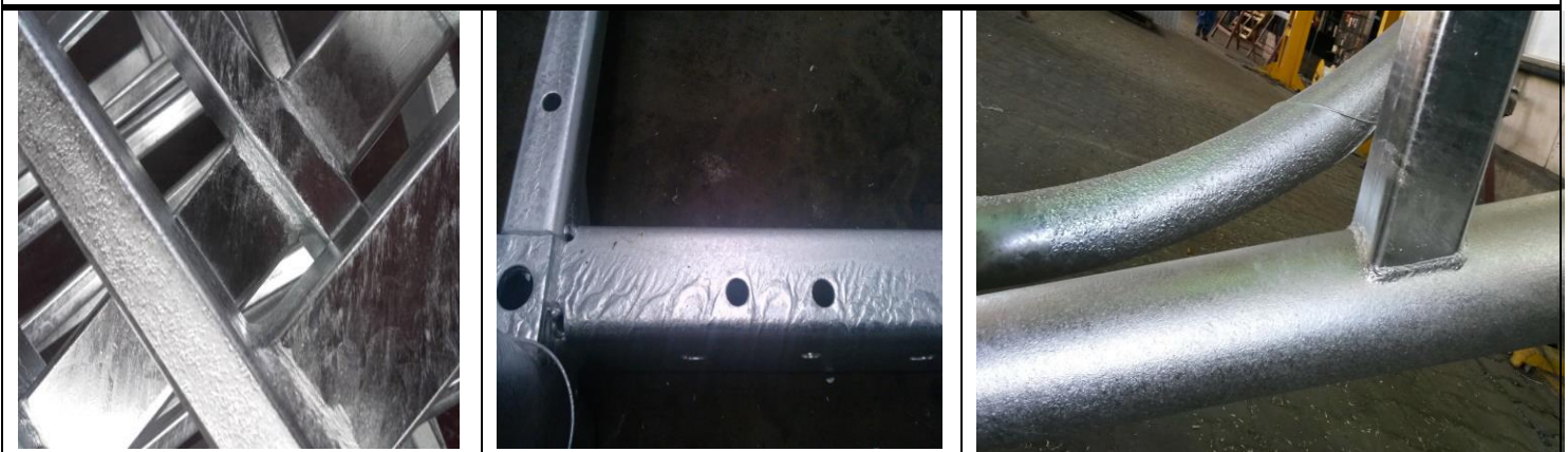
Coating structure resulting from the steel grade
