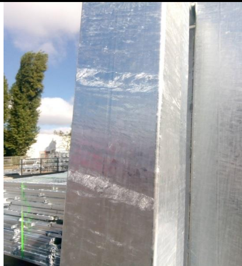
Precipitated aluminum – scum – is not removed
