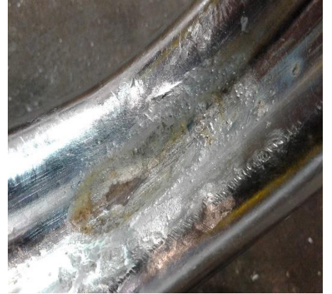
Impurities on steel, sticker marks resulting in lack of zinc plating – remain unpainted
