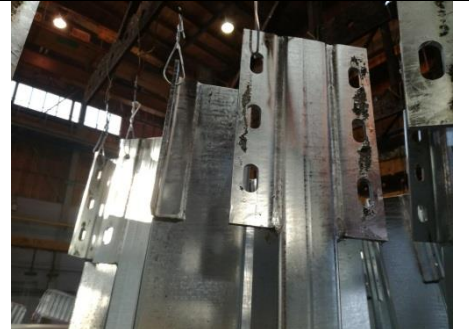
Impurities on steel, sticker marks resulting in lack of zinc plating – remain unpainted
