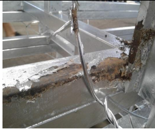
Coating to be repaired according to item 5 TAC
